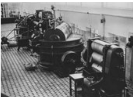
⌘ p. 58–59 FOUR-ROLL ROLLER MILL AND A COVERED LEHMANN MELANGEUR WITH A DEVICE FOR LIFTING THE SLIDERS FOR GRINDING AND CYLINDRICAL ROLLING TO OBTAIN THE EXCEPTIONAL FINENESS AND HOMOGENEITY OF THE CHOCOLATE MASS IN ISKRA IN SVOGE. THE MACHINES WERE LOCATED ON THE THIRD FLOOR (TODAY'S SPACE FOR PL16 MANUAL ARRANGEMENT).
