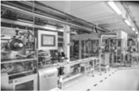
➤ p. 308 TTME MODULE ON LEKOS 3 – AUTOMATIC ARRANGEMENT OF CHOCOLATES INTO BOXES, 2022.
