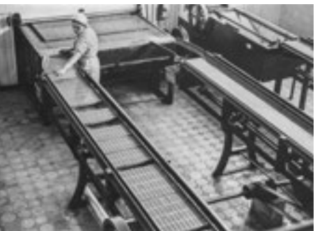
⌘ p. 70–71 THE MOULDED CHOCOLATE ENTERS THE COLD ZONE IN ISKRA, SVOGE. THE WORKER DIRECTS BY HAND FILLED MOULDS TOWARDS ONE LANE OF THE CONVEYOR BELT. THE THIRD BRANCH IN THE PHOTO IS MEANT FOR PRALINES.
