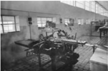
➤ p. 78–79 LOESCH LU3 MODEL 1935 PACKAGING MACHINE BY MAX LOESCH, PRODUCING 60 BARS PER MINUTE FOR OVER 50 DIFFERENT TYPES OF PACKAGING INSTALLED IN ISKRA – SVOGE (1938).
