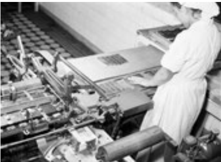
➤ p. 115 IN THIS PHOTO – THE PACKAGING STAGE OF THE CHOCOLATE UNIT. ON THE RIGHT – ISKRA’S MAX LOESCH MACHINE FOR PACKAGING CHOCOLATES.
