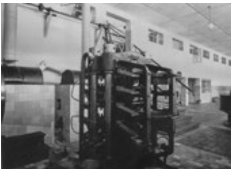
⌘ p. 54–55 VERTICAL FOUR-POT PRESS BY J. M. LEHMANN, PRODUCED IN DRESDEN, IN ISKRA FACTORIES IN SVOGE; IN THE BACKGROUND ON THE LEFT SIDE – TWO MACHINES FOR SUPPLY OF CHOCOLATE MASS INTO THE PRESS. THE PRESS ITSELF WAS LOCATED UNDER THE UNIT FOR STORING, SORTING AND BAKING THE CACAO (TODAY'S LINE FOR MANUAL ARRANGEMENT – PL16).
