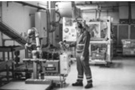
➤ p. 307 COBOTS WERE INSTALLED ON CAVEMIL AND AASTED LINES IN 2020.
