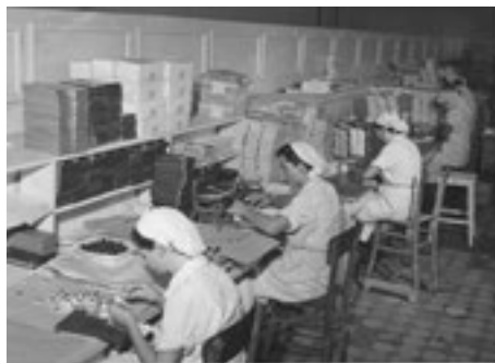
➤ p. 150–151 THE MANUFACTURING PROCESS OF HAND PACKING IN SEQUENCE: WRAPPING THE CHOCOLATES IN FOIL; BOXING AND MEASURING; PACKAGING AND LABELLING THE BOXES.
