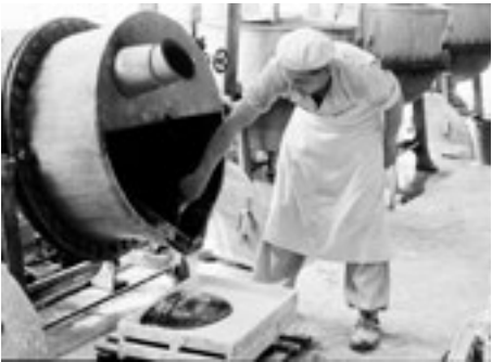
➤ p. 134–135 PRODUCTION IN THE TURKISH DELIGHT UNIT – BOILING DEPARTMENT – POURING THE FINISHED MASS FROM THE TEMPERING POT INTO THE MOULD (REUSABLE WOODEN MOULDS ARE STILL USED FOR TURKISH DELIGHT IN MANY FACTORIES TODAY). AFTER MOULDING, THE MOULDS ARE STACKED ON TOP OF EACH OTHER AND THE PRODUCT IS LEFT TO ‘MATURE’ IN A TEMPERING CHAMBER FOR 48 HOURS BEFORE BEING HAND-CUT AND PACKAGED.
