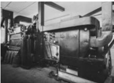
⌘ p. 52–53 MACHINES FOR PEELING AND BAKING THE CACAO BEANS AFTER SORTING (FOURTH FLOOR OF THE ISKRA FACTORY (TODAY'S MANUAL ARRANGEMENT LINE – PL16)).
