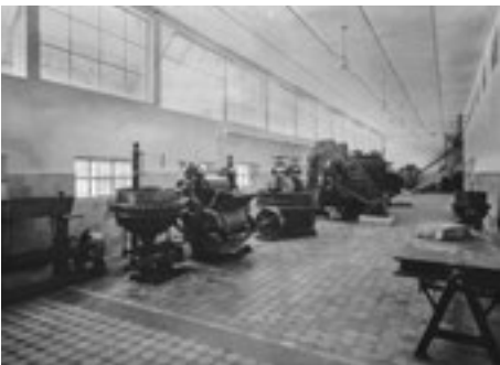
⌘ p. 60–61 PART OF ISKRA'S MACHINERY PARK (LEFT TO RIGHT – A FONDANT MACHINE, A CHOCOLATE TEMPERING MACHINE (FOR PRALINES), A ROLLER MILL AND A COVERED AND UNCOVERED MELANGEUR. IN THE BACK BY THE STAIRS IS THE PRESS FOR COCOA BUTTER. ON THE RIGHT SIDE ON THE SPECIAL METAL TABLE IS PART OF THE 'CAKE' OF PRESSED COCOA.
