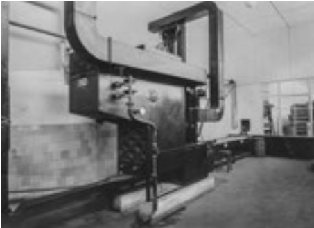
⌘ p. 50–51 A BUNKER IN ISKRA FACTORY, IN WHICH CACAO BEANS ON THE TRANSPORTATION BELT ARE SORTED MANUALLY BEFORE GOING INTO THE MACHINE FOR SORTING AND CLEANING.
