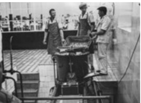
⌘ p. 68–69 A DEPOSITOR BEING MANUALLY FILLED WITH CHOCOLATE MASS FOR MOULDING IN ISKRA FACTORY – SVOGE. IN FRONT OF IT IS THE MOULDING PRODUCTION LINE. THE CHOCOLATE TO FILL THE MACHINE WAS CARRIED BY HAND IN METAL CONTAINERS.
